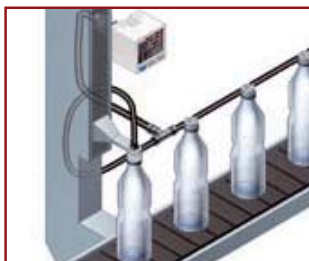
Air-leak test for PET bottles
